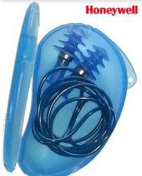
Reusable insert detectable from metal detector. The soft dual material gives perfect comfort. Quadruple soft flange for better conformation of auditive channel. Rigid rod for an easy fitting. Detachable cord, for safety matter (catch). Practical case. Washable and riusable for 2-4 weeks. dedicated to food industry SNR 28 DB
