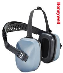
Thanks to the patented Sound Management sound filtration technology. They allow the user to hear the voices of other workers, alarm signals in a more natural way, blocking at the same time the harmful noise. Dielectric version. Snap-on bearings. The multi-position headband allows the user to select the position above or behind the head or under the
