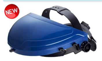
Without metal parts for electric arc protection. Front sweatband in interchangeable sponge, upper band for adjusting the height of the shell, cranial adjustment through rack (from 53 to 61 cm), tilting by 90 ° with clutch (screen Art.UNI.69999000 transparent). EN EN 166, EN 167, EN 168, EN 170, EN 175.
