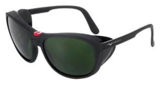
Black frame, 5 DIN green lenses in scratch-resistant polycarbonate with side protections. Protects against impacts, UV rays, infrared rays (IR) and glare generated by welding processes.
