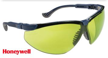
Wrap-around lens with 9 points of curvature, with anti-scratch treatment. For protection against moving particles; impact resistance test. To be used as a support during welding and brazing work. Suitable for welding assistance work, not suitable for welding and oxy-fuel work. Lens marking 1.7 B - D 1 FT. EN 166/169/175.
