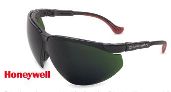
Polycarbonate lens wrapped at 9 bending points; C / antigraphic treatment. Adjustable brackets ,bend and extensible. Suitable for: Gas welding: Acetilene flow <70 liters / hour, Oxygen flow <900 liters / hour, Arc welding: Flow <6 A, Microplasma welding: Flow <6 A. Lens marking 4 B - D 1 FT . EN 166/169/175
