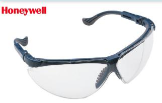
Polycarbonate lens wraparound with 9 points of curvature; with anti-scratch treatment. Adjustable temples. Soft hake. Arcade equipped with a soft seal to ensure perfect adherence. Ideal for protection against mechanical risk, for example: grinding, turning, milling, woodworking, etc. UV protection.
