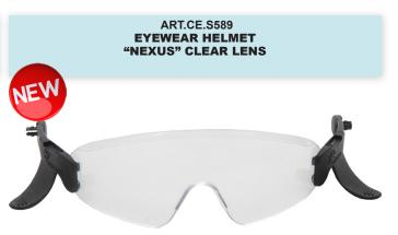
Replaceable and easy to assemble eyeglasses with anti-scratch / anti-fading lining, with curtain ascent and descent for the helmet, in combination with the helmet it can be used in explosive atmospheres as it provides antistatic protection, according to IEC 60079-32-2: 2015 electrostatic risk tests. These products have been designed to last up to 5 years. One size. Color: clear. Standards: EN 170 2C-1,2, EN 166 F1, ANSI / ISEA Z87.1-2015.
