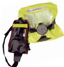
The hood OPENGO ABEK1 P3. Consisting of: hood in coated fabric, panoramic visor, filter for organic vapors (solvents), inorganic gases (chlorine and hydrogen sulphide, ammonia, powders). Complete with bag to adapt to the belt. Neck seal in flexible elastomer. The maximum storage time is 10 years, if stored in original packaging without damage. Keep the cap away from direct light and dust by keeping it in its original packaging or sealed.
