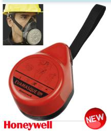
Shaped half-mask in black EPDM, elastomer harness, silicone and neoprene valves, ABEK protection. Packaged in rigid, sealed case. Practical and simple: safe to use, easily attachable to the belt. Storage up to 12 years: (4 years without maintenance). Fields of use: evacuation in case of accidental spills of liquids, chemical industry and petrochemicals.
