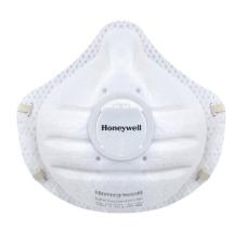
Filtering face, in hypoallergenic material. Without preformed nose clip to use without any adjustment. Its concave shape widens the field of vision and allows you to wear safety glasses comfortably. Double elastic fixed with staples.
