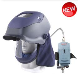
Airvisor 2 W Series for welding, complete with: High temperature resistant mask, 110 x 90 screen, internal visor with PC screen, flame retardant fabric lining, belt with filter (DAVW-1003E) with alarm and bag for storage.
